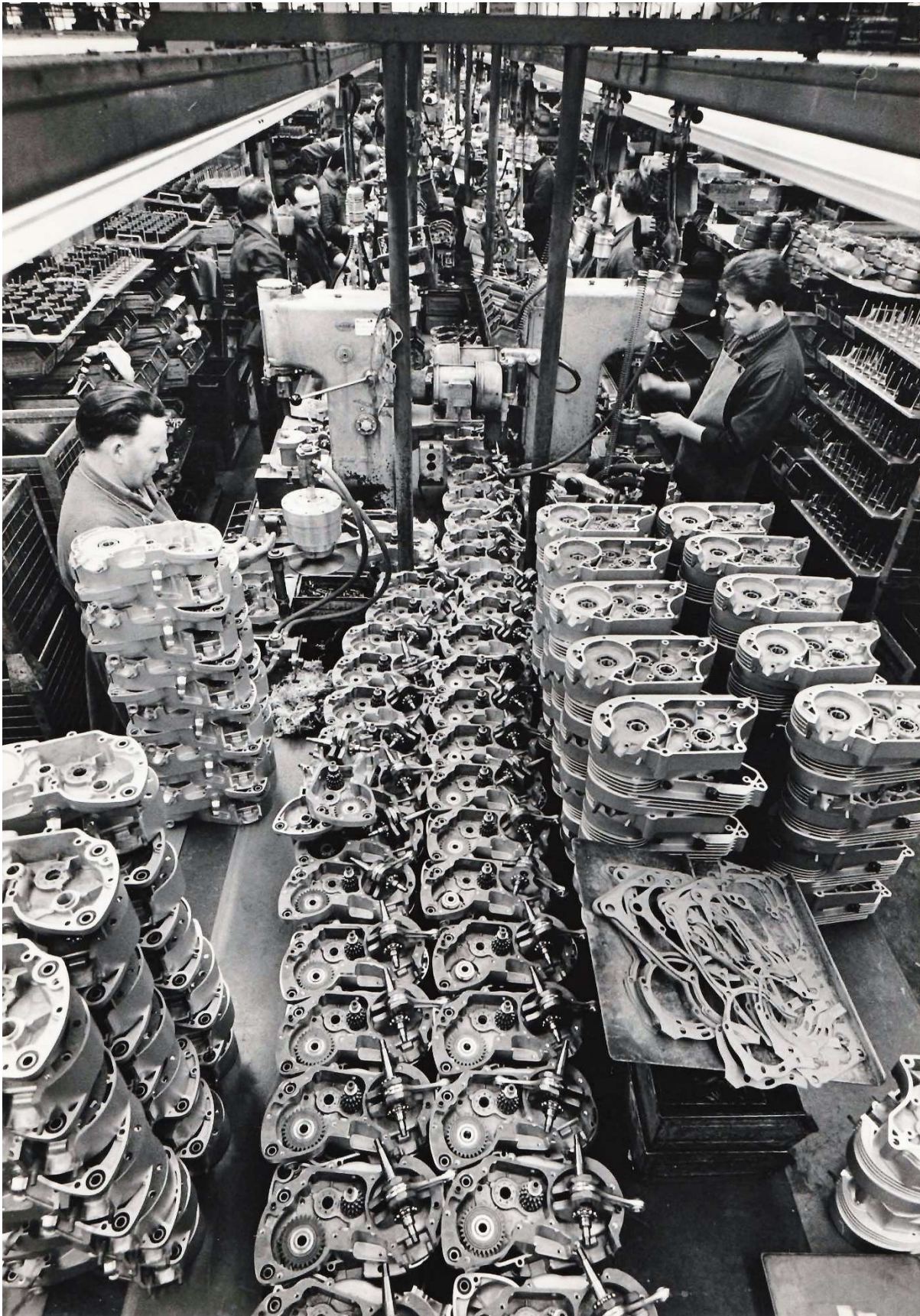
Assembly line in 1966 showing assembly process on an engine very similar to the Messerschmitt 200AZL-R. Note that the cases are not matched pairs but are marked with an assembler ID number on completion. Photo: MFGB archive.
